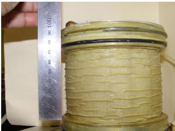
Figure 5: Uniform deformation of the specimen during shearing up to a large strain of \varepsilon_1 > 30\% .
